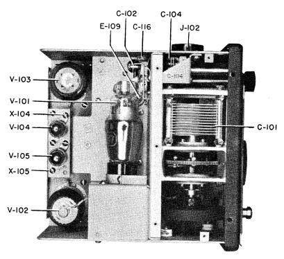
Figure 12. Top View of Chassis, Condenser Shield Removed RESTRICTED
