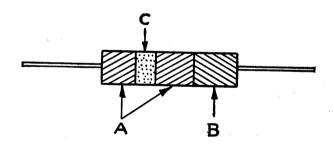
The body (A) of the resistor is colored to represent the first significant figure of the resistance value. One end (B) is colored to represent the second significant figure and a band, or dot (C) of color, located within the body color, indicates the decimal multiplier.
