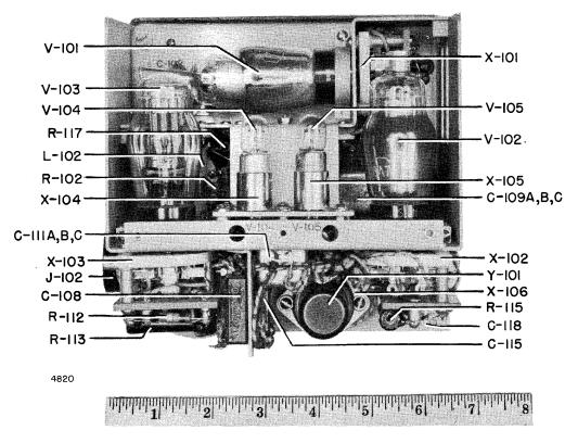
Figure 6. Rear View of Chassis (Model with Crystal Trimmer)
