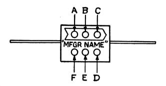
Dot A indicates the first significant figure of the capacitance of the capacitor.
