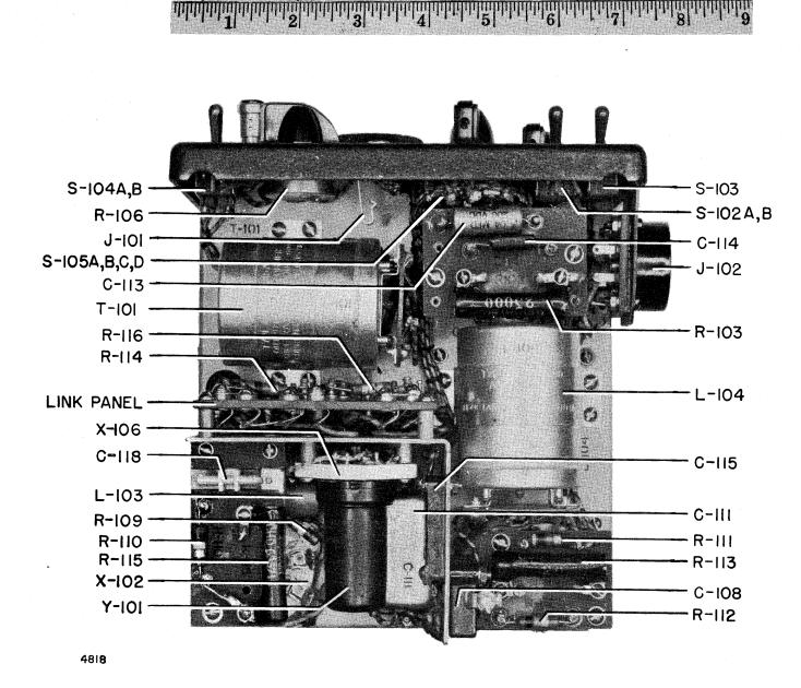
Figure 14. Bottom View of Chassis (Model with Crystal Trimmer)
