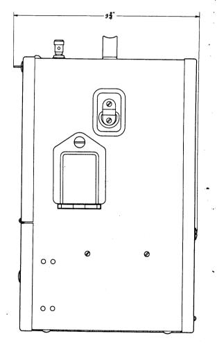
WEIGHT OF CASE WITH TYPE CRR-14028 FREQ. METER WITHOUT BATTERIES 25.5 LB3. WEIGHT OF CASE WITH TYPE CRR-14028 FREQ. METER AND WITH BATTERIES 38.9 LB3.
