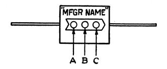
Dot A indicates the first significant figure of the capacitance of the capacitor.
